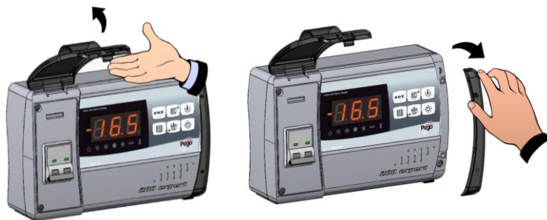
Fig. 1: Lift the transparent door that protects the differential magnetothermal circuit breaker and remove the cover for the screws on the right side.
