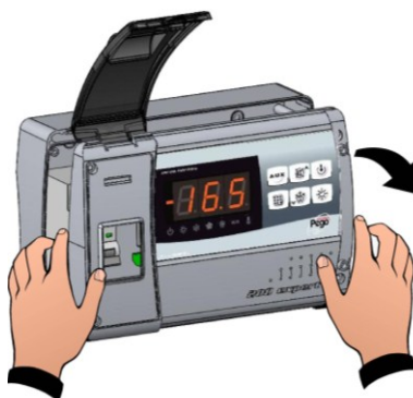
Fig.4: Open the front panel of the box by lifting it and sliding the two hinges until they reach the end stop.
